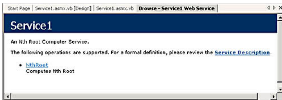
Figure 13-1. The default test interface for a Web service exposes links for launching the Web methods.
