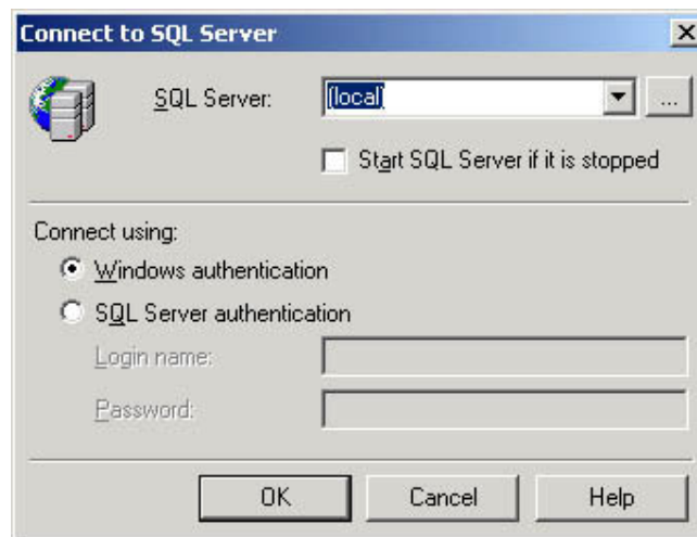
Figure 1-9. The connection settings for logging in to the local instance of SQL Server with Windows authentication.
