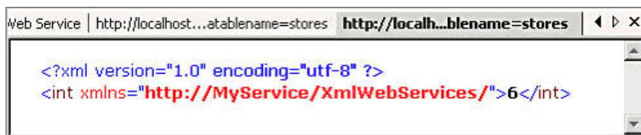
Figure 13-9. The XML returned by the RowCount Web method for the Web service in the TableProcessor folder with pubs as the database name and stores as the table name.
