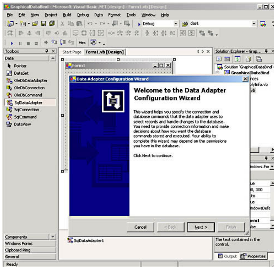
Figure 1-5. The Data Adapter Configuration Wizard enables you to graphically configure a SqlDataAdapter object and its related SqlConnection object for use with a Windows form.
